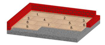
GUTEX Thermosafe-wd installs in offset joint arrangement. Use the oddment of the last board of a row to start the next row (refer to layout plan).
